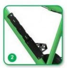
Install the base plate on the electric bicycle
